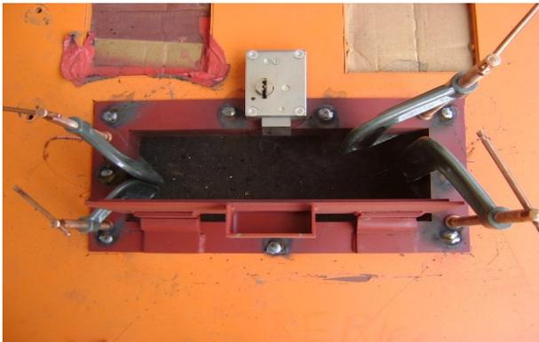
Be sure to securely clamp the two halves together as you continue to tack weld the assembly to the door.
