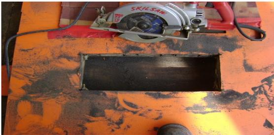
Start your third step in this process by drilling the corners of your cut with a 1/4" drill bit. Proceed by making your cuts. I use a worm drive Skill Saw with a 7"x1/8" x DM-16mm Norton metal cut off blade part 89097. The door may need to be flipped and cut on the other side. Use your 1/4" holes as a guide.
