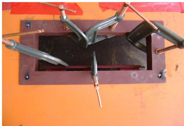
The inside trim ring should line up correctly with the front door assembly. You can weld these two together if you plan to go back and grind the weld flush.
