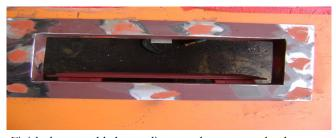
Finish the assembly by sanding any sharp or rough edges. Tape the door off and paint.
